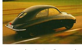
plane wing. In spite of its compact, aerodynamic exterior, it was remarkably spacious inside. In the front, there was a small but energetic two-stroke, two-cylinder engine. It was transversely mounted and drove the front wheels, thereby providing more space and driving safety for the occupants.
